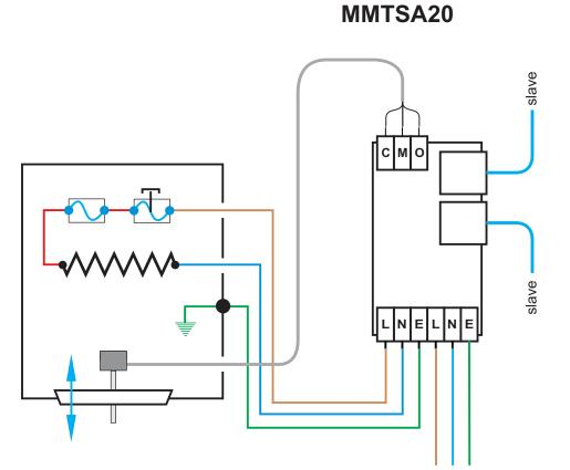
NOTE: The above slave unit functions with the MMTM master controller only.
